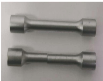
图 3 铍材试样断裂前、后的宏观形貌 Fig.3 Macro morphology of beryllium samples before and after fracture
